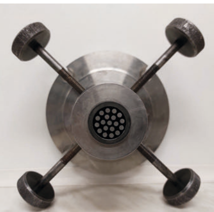
Extrusion tool for the shaping of the green bodies.
